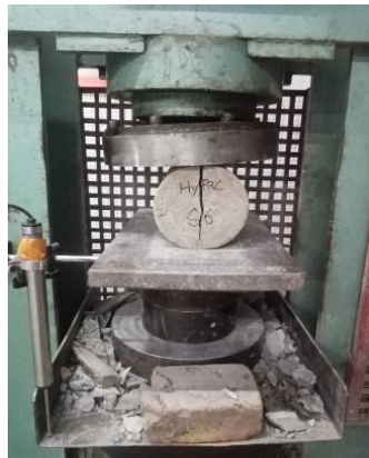
Figure- 16: HyFRC-S6 Cylinder after split-tensile strength test
