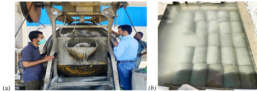
Figure- 2: Casting and Curing of Specimens (a) Preparation of Concrete mixing in Plant (b): Placement of concrete cylinders inside curing tanks for 28 days
