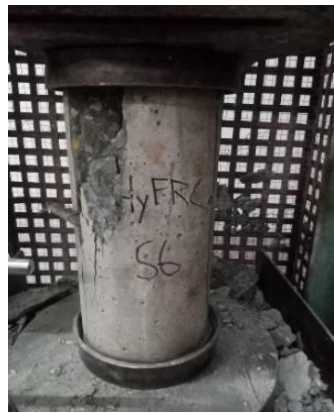
Figure- 13: HyFRC-S6 Cylinder after compressive strength test
