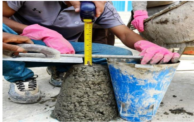
Figure- 11: Slump Cone Test for concrete specimens
