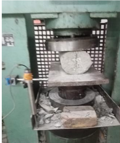
Figure- 18: Controlled Concrete Cylinders after split-tensile strength test
